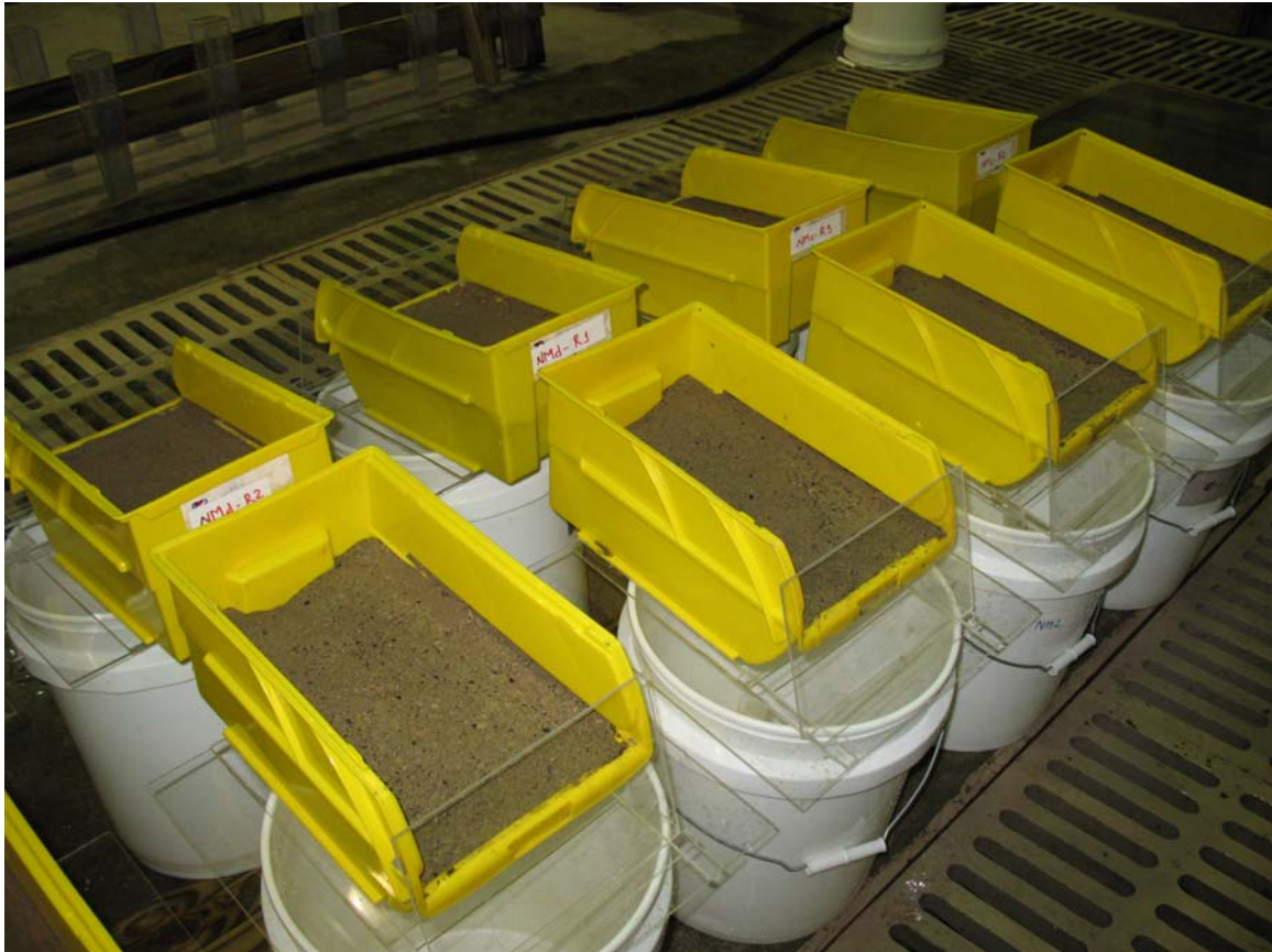
Figure 25: Rainfall Simulator – Soil Samples (details)
