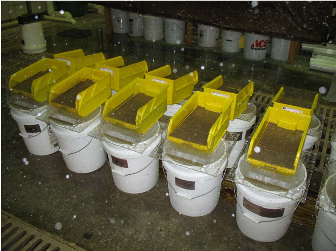
Figure 24: Rainfall Simulator – Soil Samples
