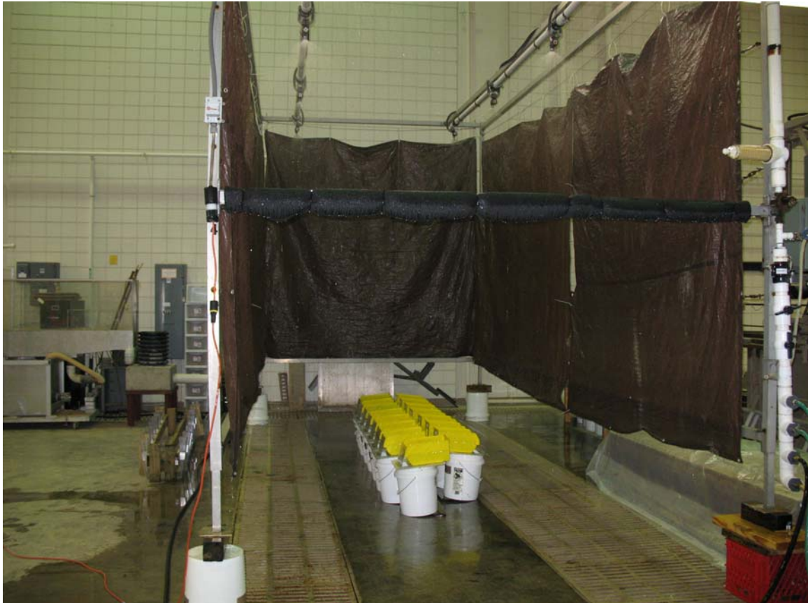
Figure 23: Rainfall Simulator – General View
