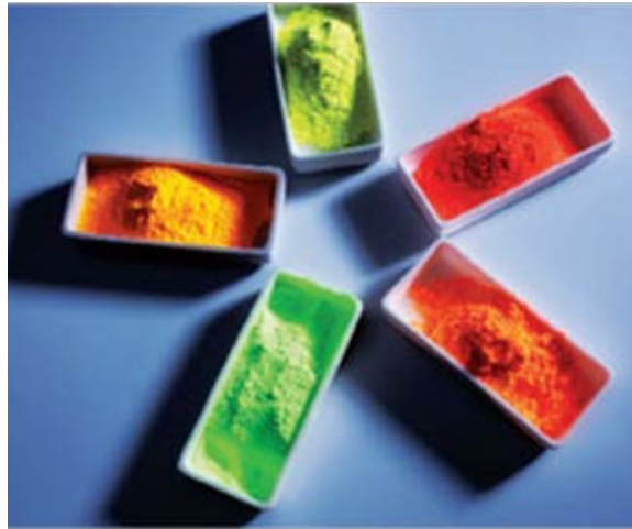
Figure 2-9. Examples of LED phosphors available at Intematix Corp.
