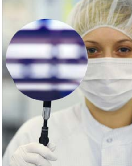
Figure 2-4. GaN-based LEDs on a 200 mm silicon wafer as demonstrated by OSRAM
