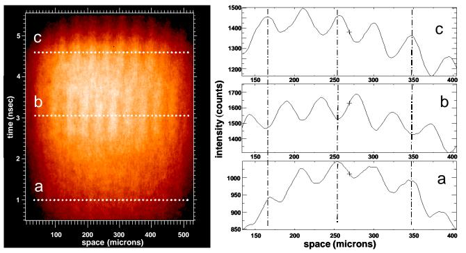
Streak record (left) and its lineouts at three different times (right) for target thickness 60  $\mu$ m,  $l = 46 \mu$ m, and peak laser intensity 5×10<sup>13</sup> W/cm<sup>2</sup>. Two phase reversals are clearly seen on both images.
