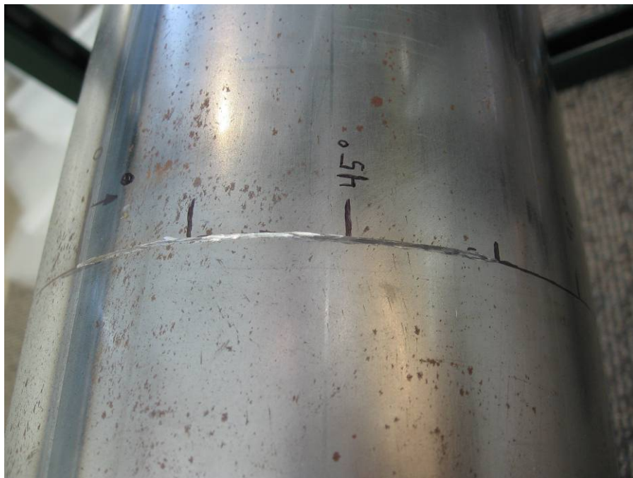
Figure 5.3: Circumferential notch, 50% through thickness, 0.0^\circ to 67.5^\circ
