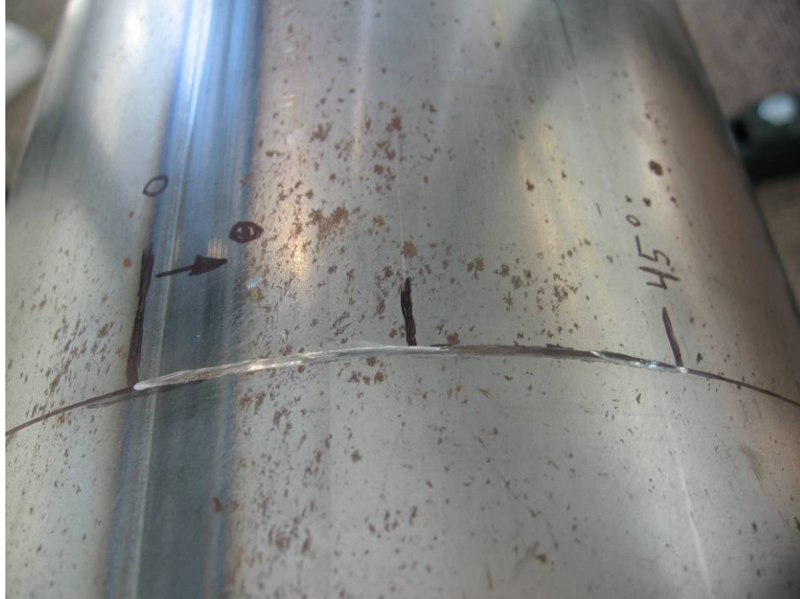
Figure 5.2: Circumferential notch, 50% through thickness, 0.0^\circ to 45.0^\circ
