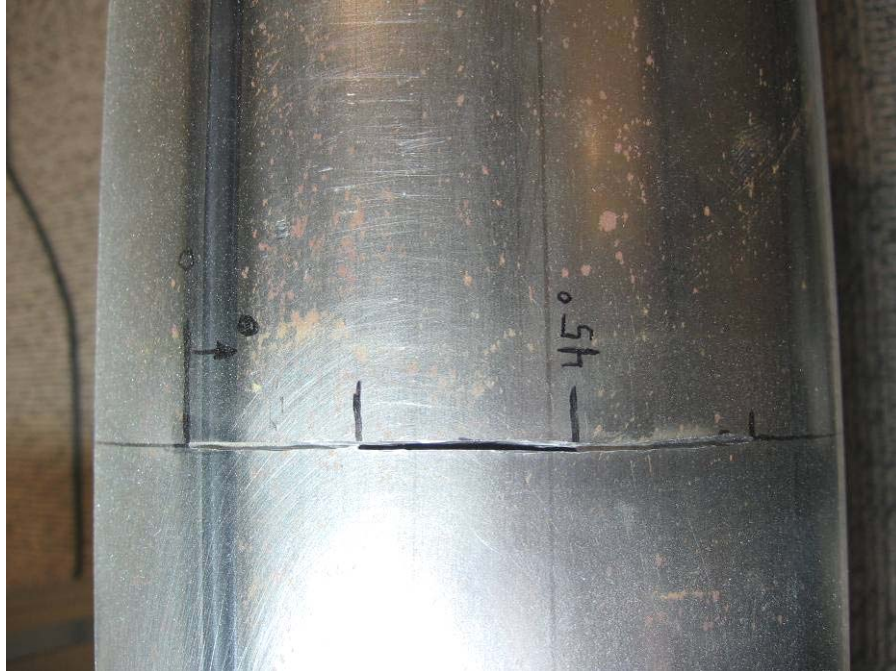
Figure 5.5: Circumferential notch, 100% through thickness, 22.5° to 45.0°
