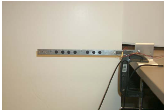
Figure 5.2 Photo of the experimental beam-mass setup.
