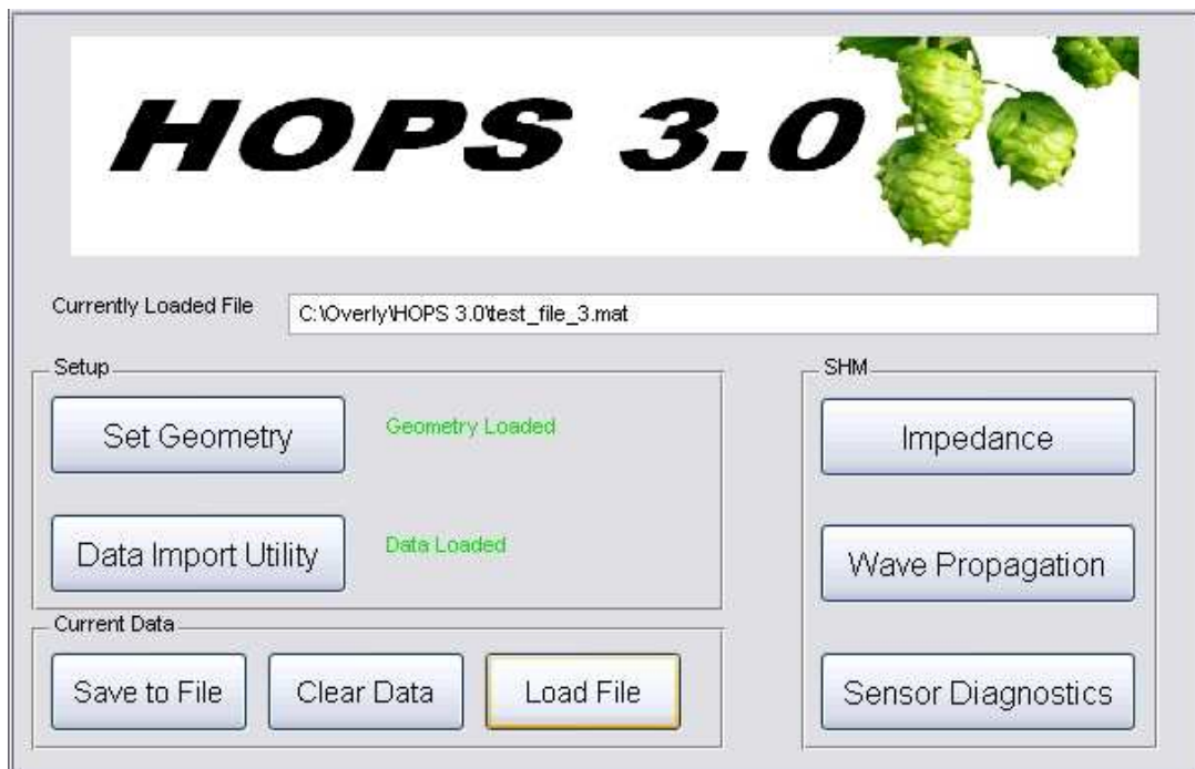
Figure 6.1: The main HOPS module now gives important user feedback with regards to file information
