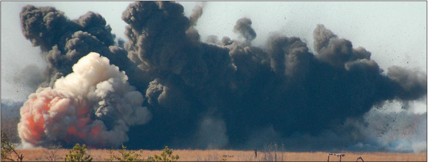
The explosive force of the Mine Clearing Line Charge (MICLIC) is used to clear paths through mine-laden terrain.
