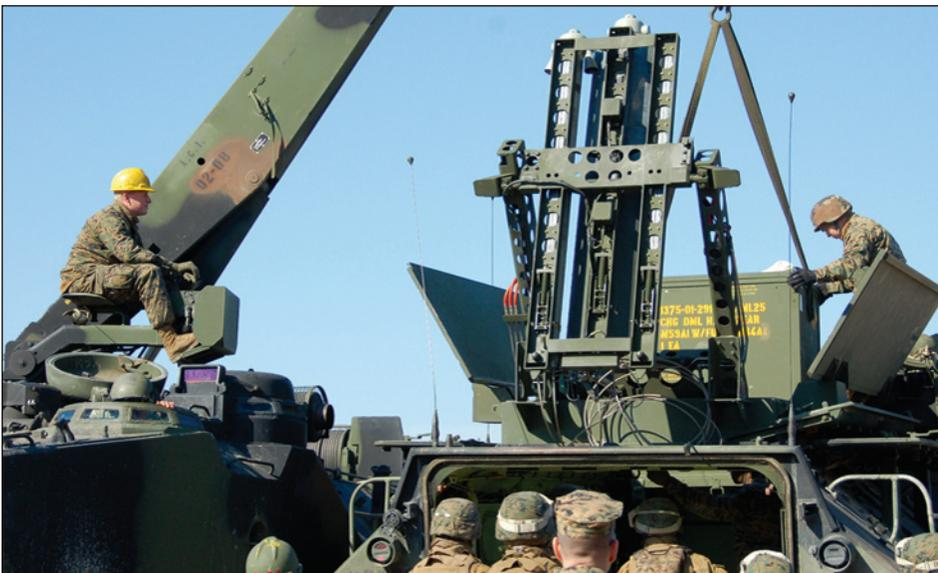
With the help of a crane, the Marine crew loads a MICLIC pod into their amphibian assault vehicle.
