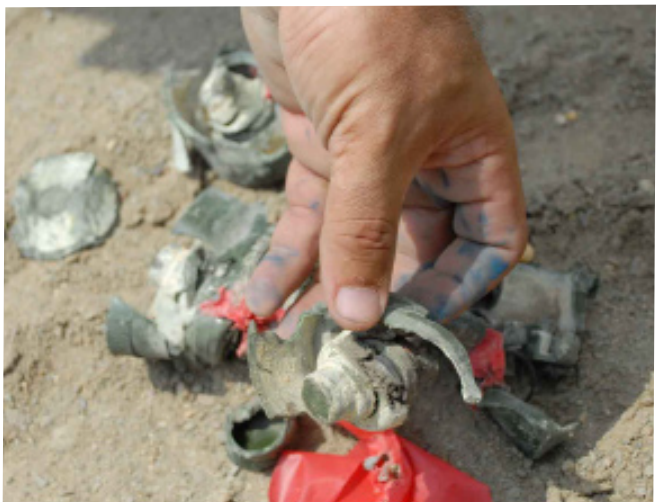
The designed end result produces pulverized safe mine components that are completely safe. (Photo by Christopher B. Joyner)
