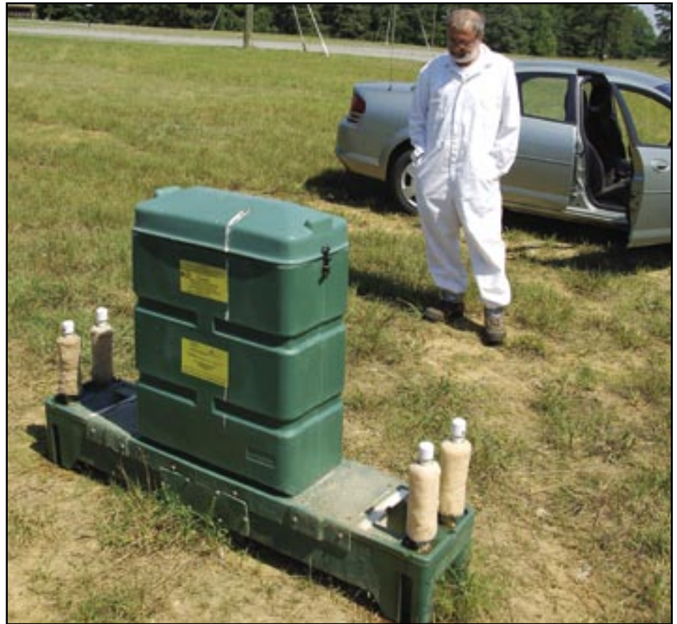
Karl Neidhardt inspects one of the many “4-poster” deer treatment devices located on Fort A.P. Hill. It places tick repellent on deer that may feed there. (Photo by Jason B. Cutshaw)
