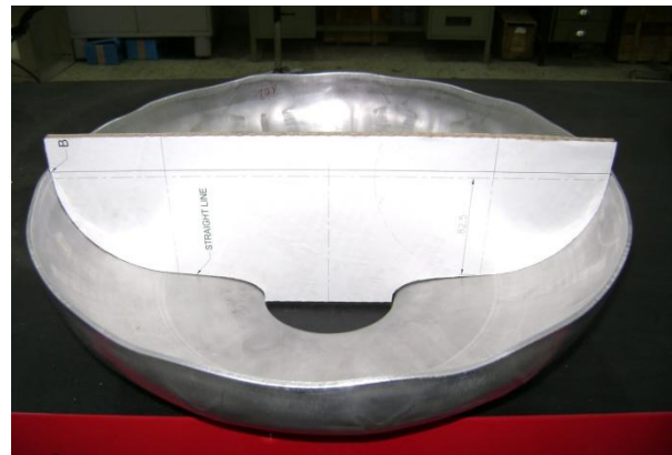
Figure 6: Half cell inspection using template
