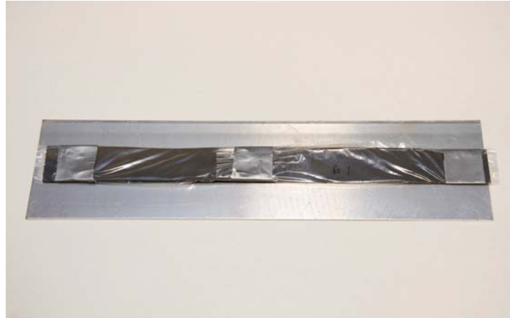
Figure 4: DU-10Mo Foil Prepared for Packaging with Hard-Back Fixture
