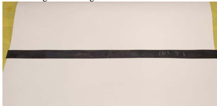
Figure 3: DU-10Mo Foil after Final Shearing Operations
