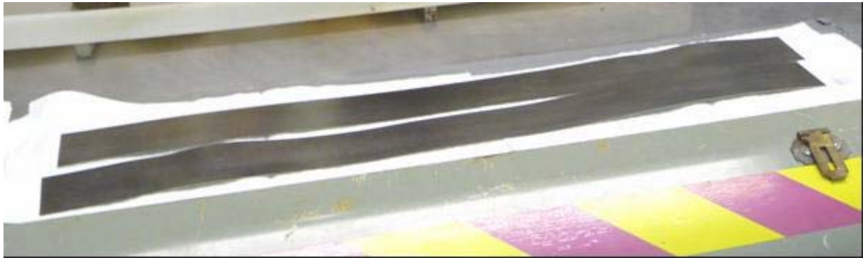
Figure 8, Polished Zr co-rolled U10Mo fuel foils ready for cladding application.
