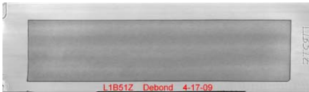
Figure 10. UT Debond scan images of AFIP-4 fuel plate sample.
