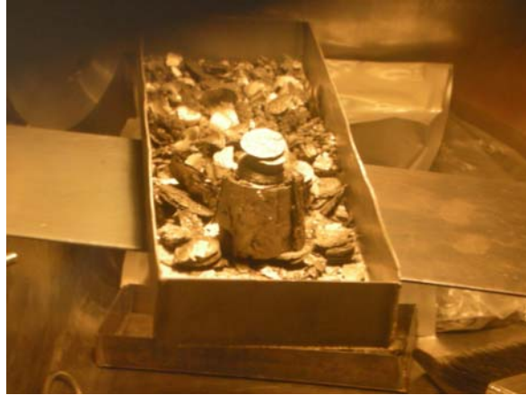
Fig. 3 The appearance of U-Mo alloy ingot after hydrogenation
