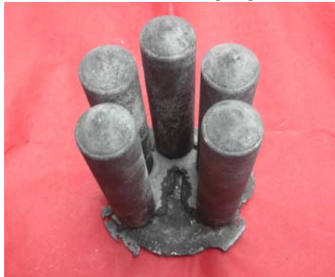
Fig. 1 The picture of casting U-Mo alloy ingot
