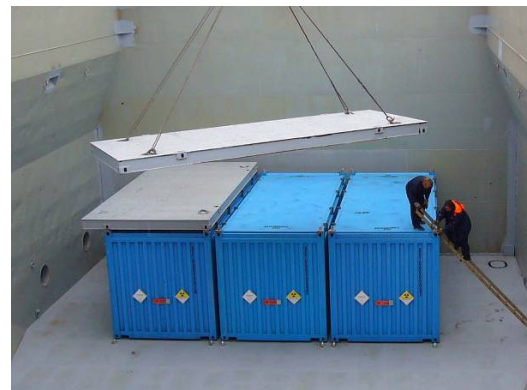
Fig. 6. Transport overpacks are loaded into the hold of "MCL-Trader" vessel
