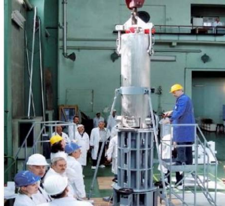
Fig. 12. Tests of the transfer cask for loading SFA into TUK-19
