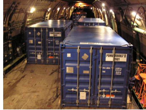
Fig. 4. Transport overpacks loaded into the cargo section of AN-124-100 aircraft
