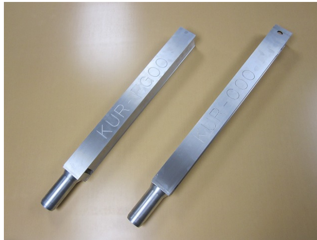
Fig.3 A standard fuel element (left) and a special fuel element (right)
