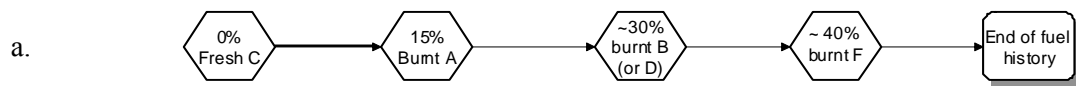
Figure 3. a. Schematic view of irradiation history of a standard BR2 fuel element, following typical reloading BR2 strategy.
