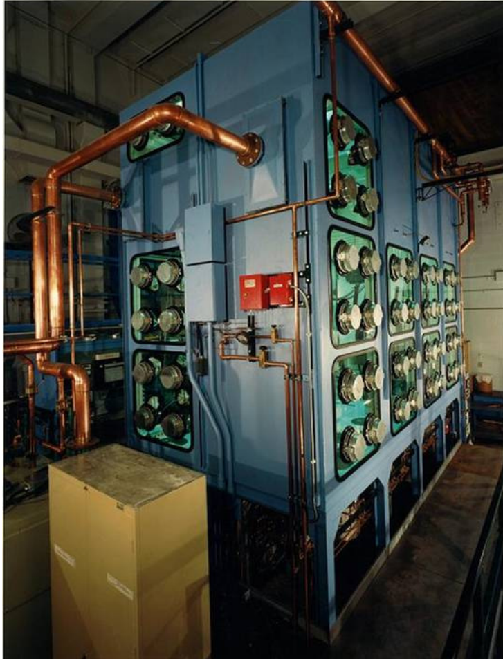
Figure 8. Engineering-Scale Glovebox Prototype
