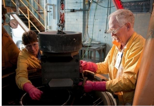
Figure 4: Removal of Mold from Furnace
