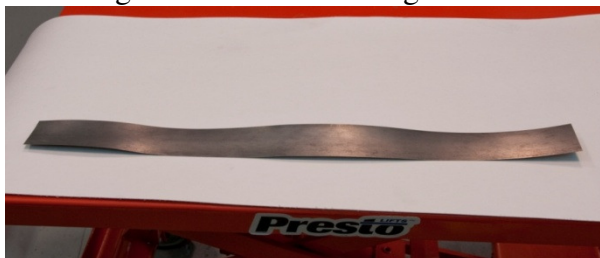
Figure 7: First Co-rolled Foil Fabricated at Y-12
