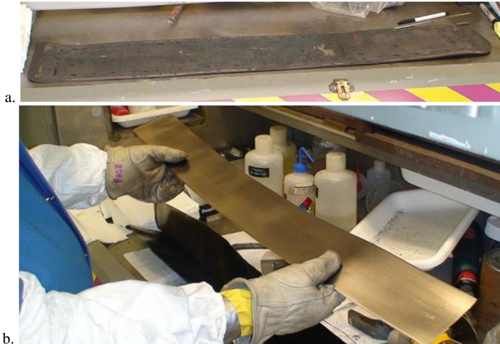
Figure 5. a) Heat treated co-rolling assembly, b) Full size Zr co-rolled U10Mo fuel foil (~85 mm x 750 mm x 0.5 mm).
