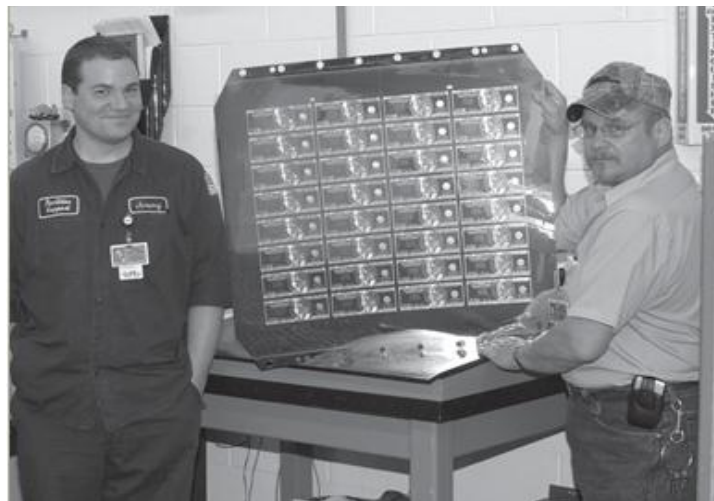
James (Jim-Bob) Thompson, Intaglio Plate Maker Foreman, shows Jeremy Clemons, Pipefitter, a 32 subject intaglio currency plate during the Office of Engraving open house.
