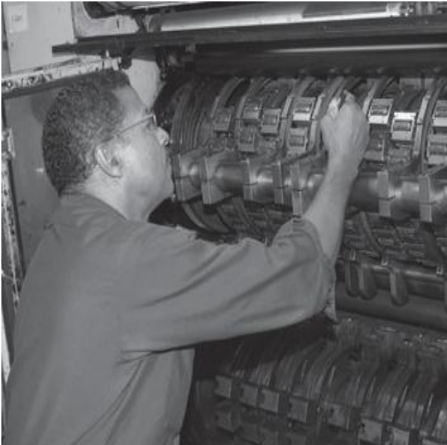
Alvin Mitchell, Cope-Pak Pressman, resets serial numbers on the currency overprinting equipment.
