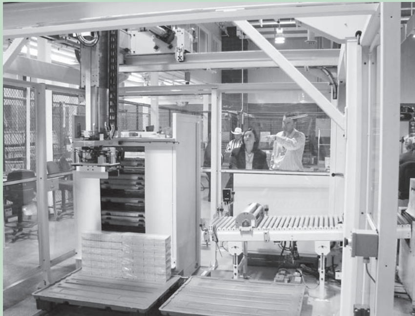
Robert Pettit, Office of Currency Manufacturing, discusses features of a new robotic currency palletizer to Treasurer Cabral.
