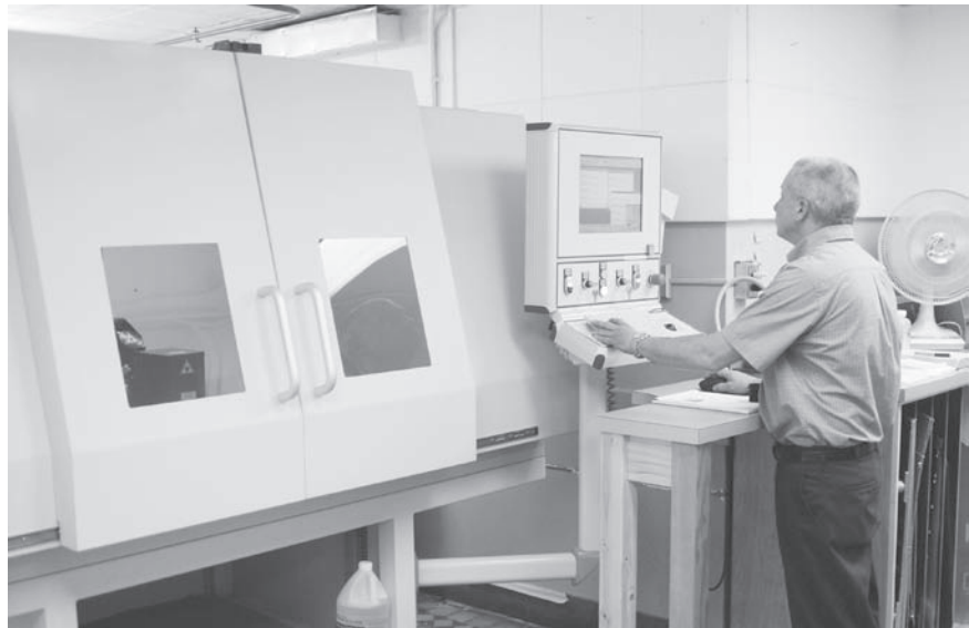
Allen Pipes, Office of Engraving, uses the new Laser Pantograph, which utilizes laser technology to etch images faster and more consistently.
