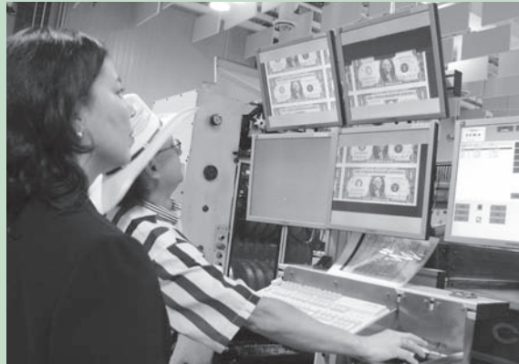
Jimmy McCollum, Electro-machinist, demonstrates the capabilities of the new Overprinting Inspection System in Fort Worth to Treasurer Cabral.
