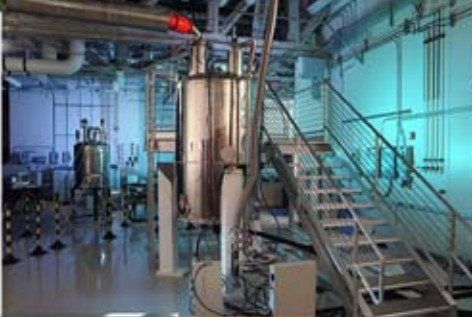
Environmental Molecular Sciences Laboratory's 800-MHz nuclear magnetic resonance spectrometer at Pacific Northwest National Laboratory
