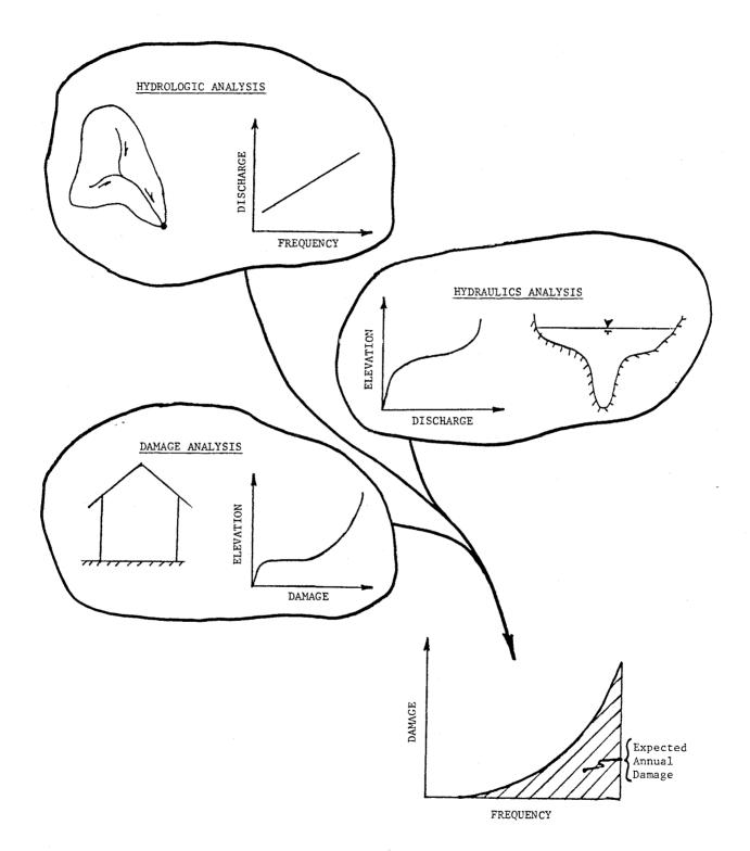
FIGURE 1 FLOOD DAMAGE ANALYSIS PROCESS
