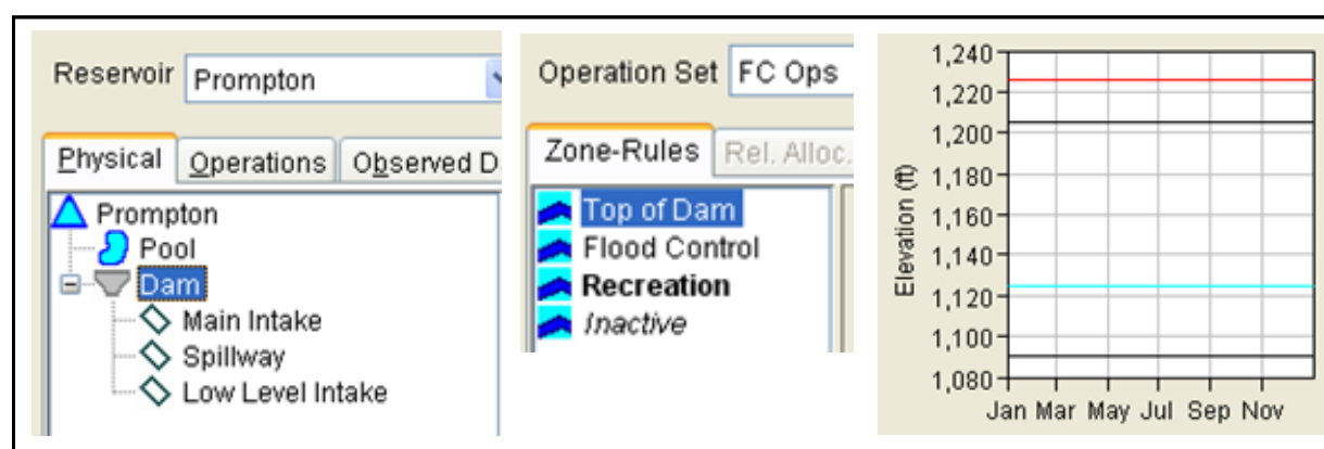
Figure 4.22 Prompton's Pool and Dam Elements and its "operating" zones
