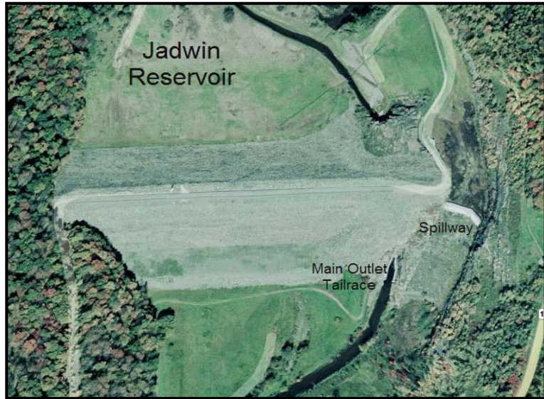
Figure 4.23 Jadwin Reservoir, a dry dam
