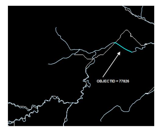
Notice how the published stream line is different than the flow accumulation grid at this location. An evaluation of the DEM, "Fill\_NoData\_2", shows a small dam at this location. In order for the GIS to create a hydrologically corrected DEM, one where the water flows across the terrain, the area behind the dam was filled in by the **Fill Sinks** tool. Filling in large areas often causes the GIS derived stream network to differ from the actual stream network.
