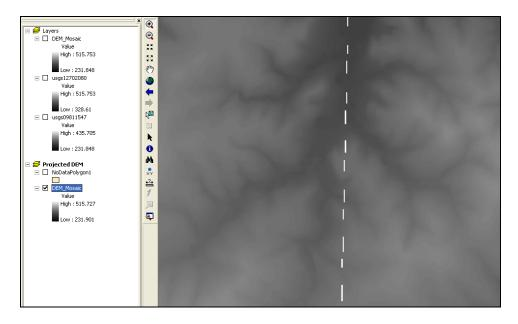
The NoData grid cells should be filled using the average elevation from neighboring grid cells.
