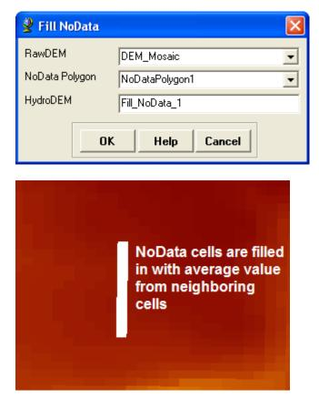
The **Identify NoData** tool should be run again to verify that all NoData cells have been filled. Six additional areas of NoData were identified in the example dataset. The **Fill NoData** tool was used a second time to fill in these grid cells. The input DEM was "Fill\_NoData\_1" and the input NoData polygon layer was "NoDataPolygon2". The output DEM was named "Fill\_NoData\_2". A third use of the **Identify NoData** tool showed no more NoData cells within the DEM.
