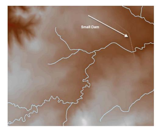
The **Fill Extent Visualization** tool will show how much of the raw DEM was filled in to create the filled DEM, "FillSinks1". This tool generates a raster showing the difference between the Filled DEM and the original Raw DEM. The resulting grid may show either the sinks or the peaks. To show the sinks, the function subtracts the Filled DEM from the Raw DEM, and changes all the zeros (i.e. identical values) into NoData cells.
