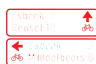
K8 Signposts (multiple) for cyclists and moped riders showing intermediary destinations and indicating an alternative route (in italics) to one of the destinations
