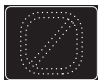
F9 End of all restrictions and advisories indicated on an electronic signalling panel
