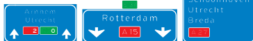
K4 High level motorway information sign showing lane instructions for through traffic and exit panel showing intermediary destinations, with the motorway number and European route numbers
