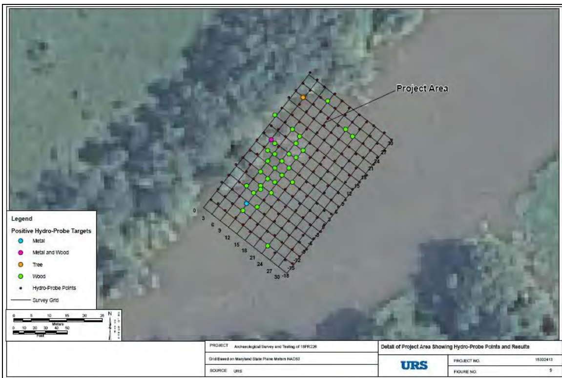
FIGURE 32. Detail of project area showing hydro-probe points and results (Pelletier et al. 2011:17).
