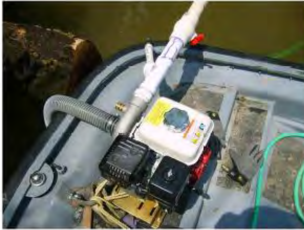
FIGURE 34. Hydro-probe pump (Pelletier et al. 2011:Fig 21).
