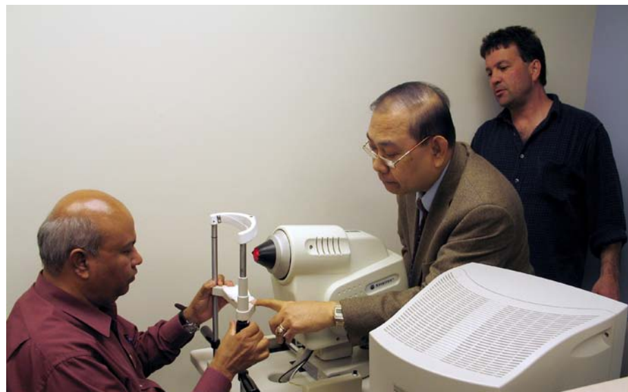
NASA's Rafat Ansari (seated) and NEI's Manuel Datiles (immediate right) working out the details of their tool that uses dynamic light scattering (DLS) to examine \alpha -crystallins, one of three lens proteins that, when denatured, allows cataracts to form. NASA technician James King looks on.
