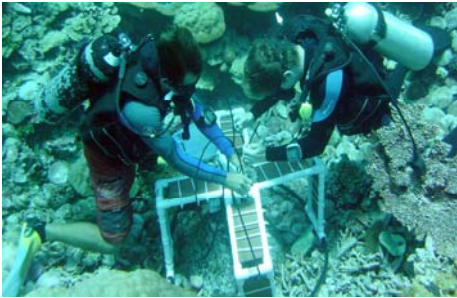
CRED divers place coral settlement plates on the seafloor to monitor coral recruitment
