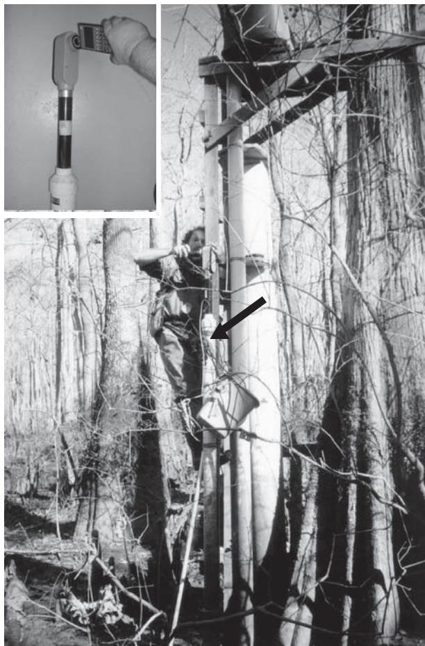
Figure 13.6. Example of an automated, single purpose water level recorder, the WL-80 being downloaded. The WL-80 (arrow) is mounted next to the stilling well of a Stevens type recorder. Inset shows the head of the WL-80 and the calculator used for downloading.
