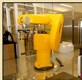
Housed at the NIH Chemical Genomics Center, these Kalypsys robots perform precision plate handling for high throughput screening. (Photo courtesy of NHGRI)
