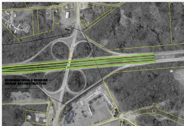
Under the NPS inside widening option, the MD 175 Bridge would require widening.
