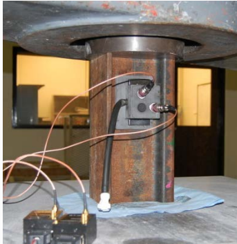
Laboratory diffuse ultrasonic measurements on rail (4 cycles)
