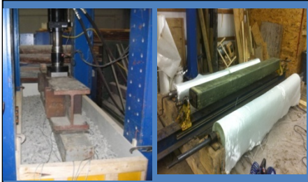
Tie with FRP shell (static bending test)
