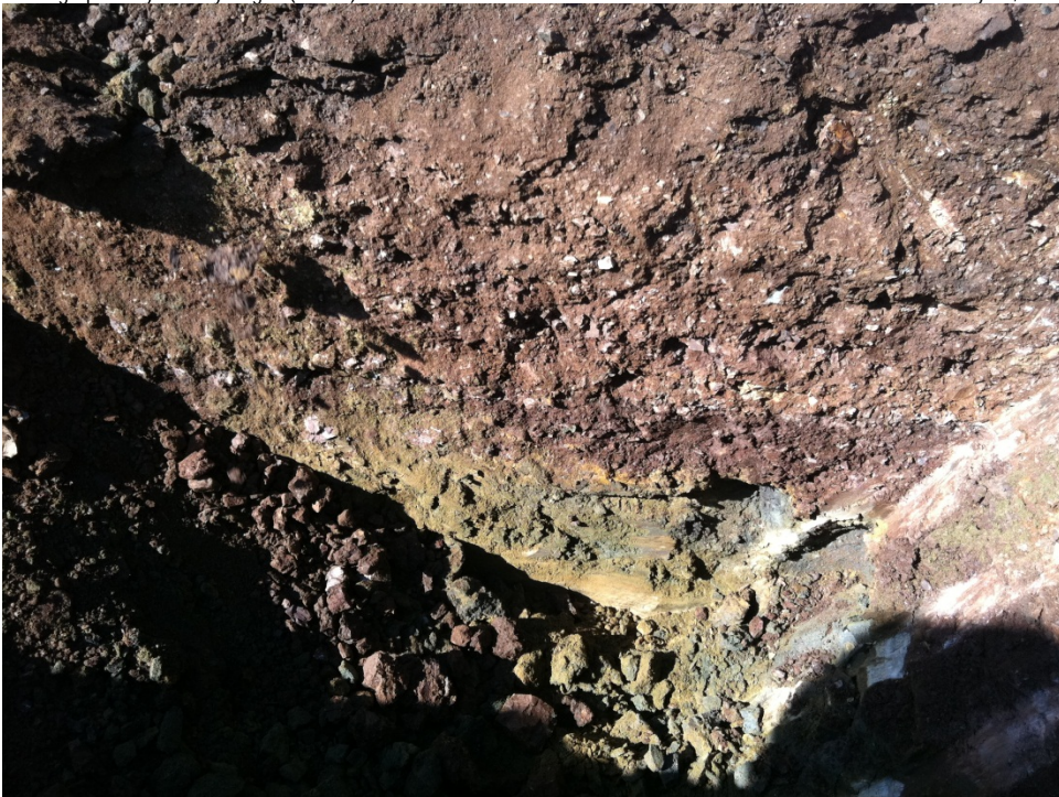
Photograph A-4: Impacted soils at 2 feet below ground surface, largest TPH stain at Fort Cronkhite Annex, facing down. .
