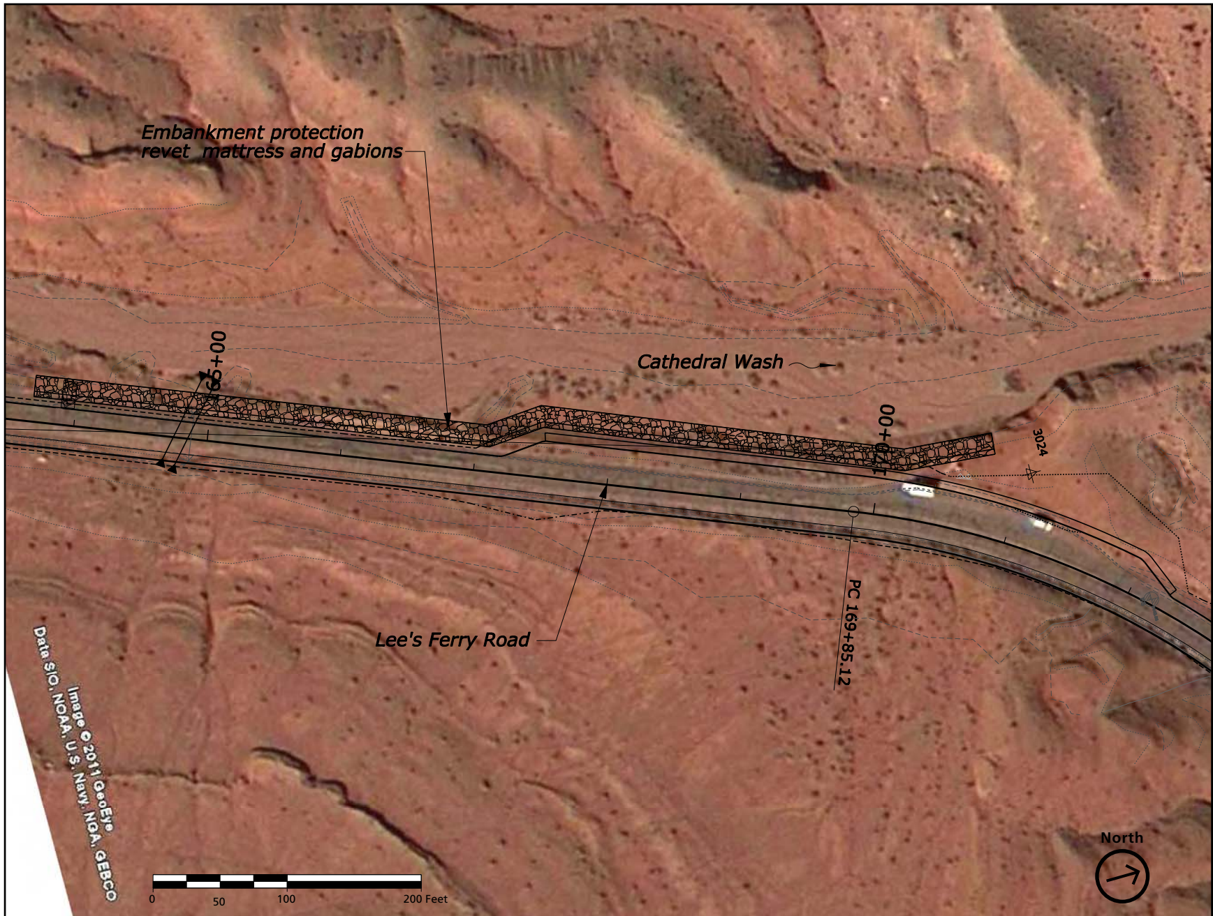
Figure 4: Cathedral Wash Bank Stabilization and Pullout Glen Canyon National Recreation Area U.S. Department of the Interior / National Park Service
