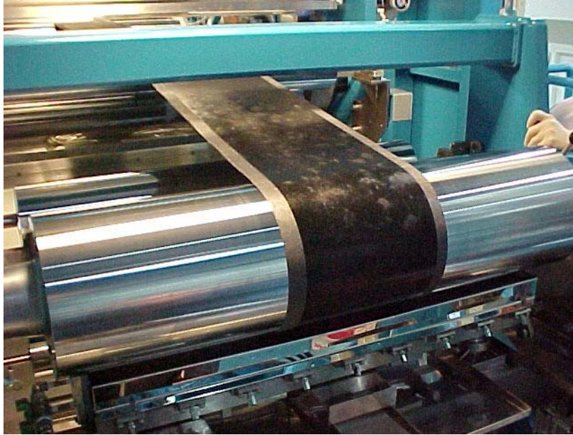
Figure 6: Semi-automated discrete/continuous fabrication of catalyst coating. 30
