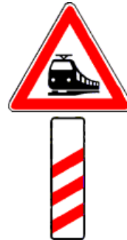
Distance to Unguarded Railroad Crossing. Indicates a crossing not separated from the road by a barrier. Posted 240 meters before an unguarded railroad crossing.
