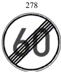
End of Speed Limit. Indicates the end of a speed-limit zone (sign 274).
