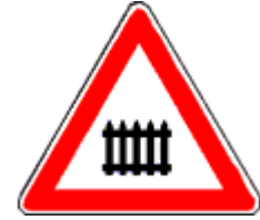
Guarded Railroad Crossing. Posted 240 meters before a guarded railroad crossing on top of the marker with three stripes (sign 153).
