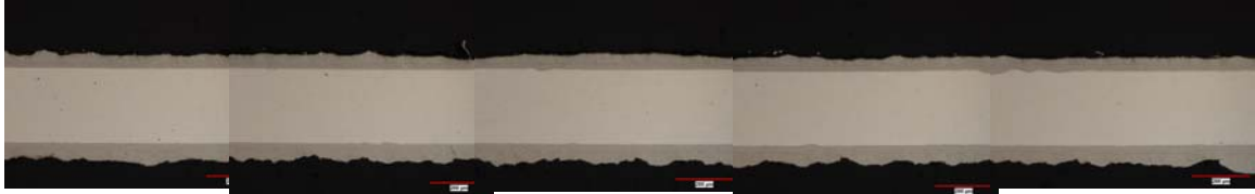
Fig. 1 Zr coating on the top and bottom of a SS substrate. The width of foil shown (the entire image width) is 4.5 mm.
