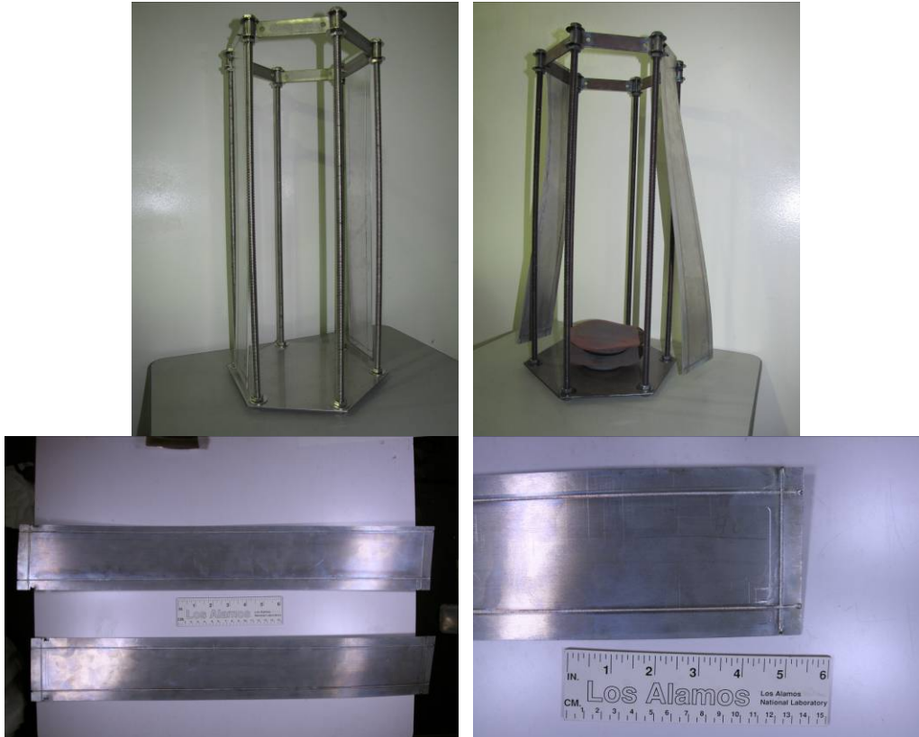
Figure 3.3. Canless foil top-mounted to HIP fixture prior to HIP processing (upper left and image) and after HIP processing (upper right image), also showing two round formed HIP cans on base plate. Lower images show plates after HIPing and details of e-beam weld. Plates are approximately 610 mm long.
