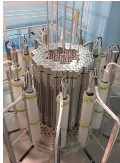
Fig.2. Critical assembly with a zirconium hydride moderator
