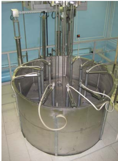
Fig.1. Critical assembly with a water moderator
