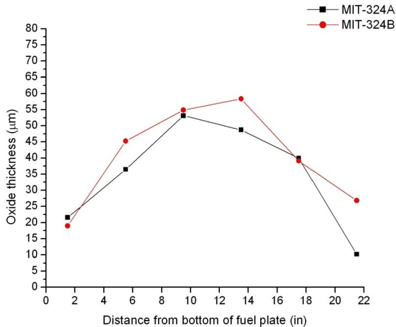
Figure 4. Results of eddy current measurements of oxide thickness on both sides of element MIT-324.
