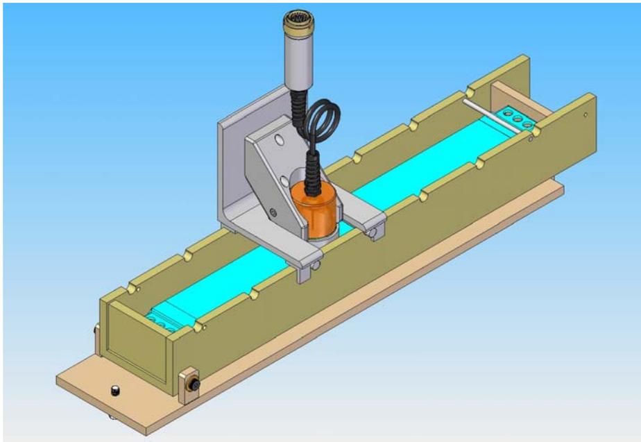
Figure 3. Fixture for eddy current and replication measurements
