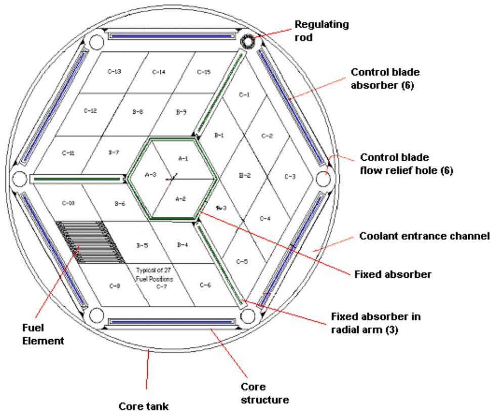
Figure 1. Layout of the MIT Reactor core.
