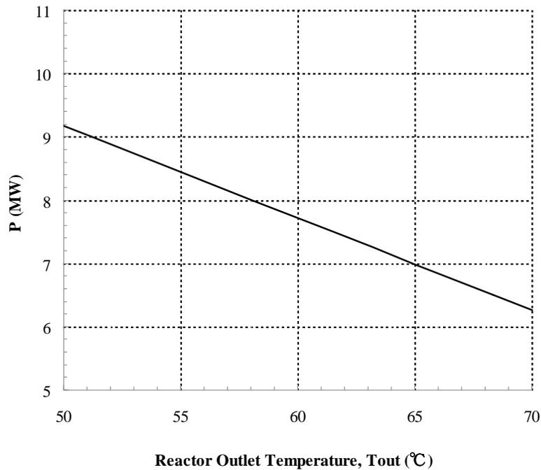
Figure 2. MITR LEU Core Limiting Safety System Settings for Forced-Flow Operation. [5]
