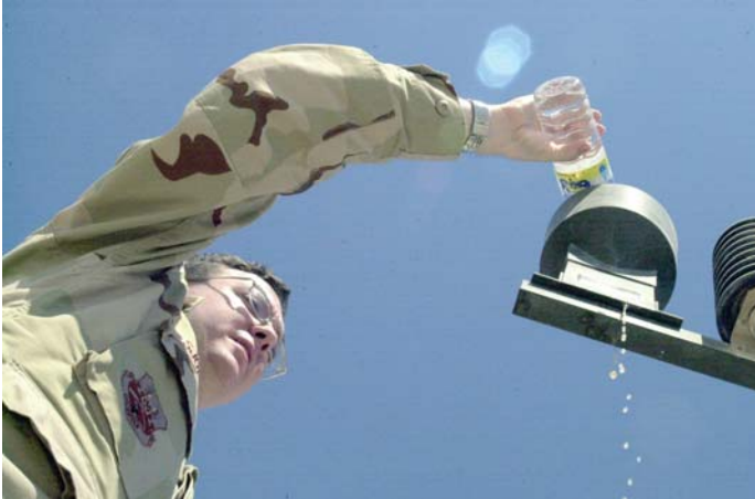
Senior Airman Jasson Sjöberg pours water into the tactical meteorological observation system as part of a function check to make sure the device, which measures precipitation, is still operational. (Courtesy photo)
