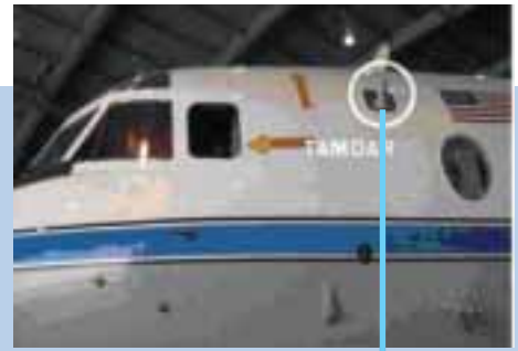
TAMDAR is designed to measure in-situ temperature, relative humidity and flight level winds.
