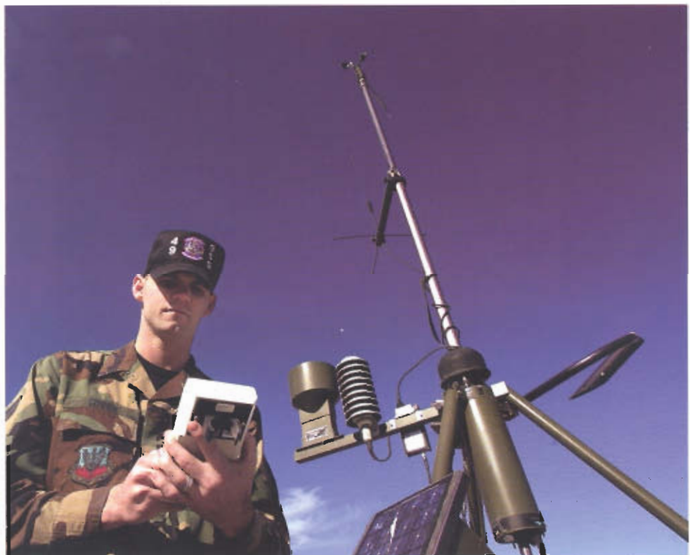
Checking the tactical meteorological observing system is one of the many duties Senior Airman Jason Conner does while working the weather desk at Holloman Air Force Base, N.M. The system is a tactical field weather station designed to be a mobile weather-gathering instrument for use in any field environment.
