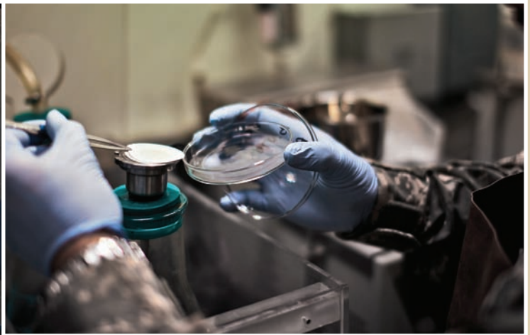
Above: After pouring a fuel sample through a filter, Spc. Juan Rodriguez-Cano, a petroleum lab technician in Company A, 615th Aviation Support Battalion, 1st Air Cavalry Brigade, 1st Cavalry Division, carefully pulls the filter off so it can be placed in an oven and later be weighed at Camp Taji, Iraq, Dec. 29, 2010.
