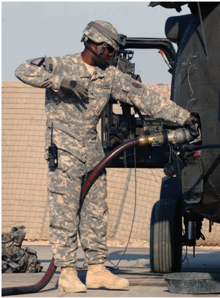
Above: After pouring a fuel sample through a filter, Spc. Juan Rodriguez-Cano, a petroleum lab technician in Company A, 615th Aviation Support Battalion, 1st Air Cavalry Brigade, 1st Cavalry Division, carefully pulls the filter off so it can be placed in an oven and later be weighed at Camp Taji, Iraq, Dec. 29, 2010.
