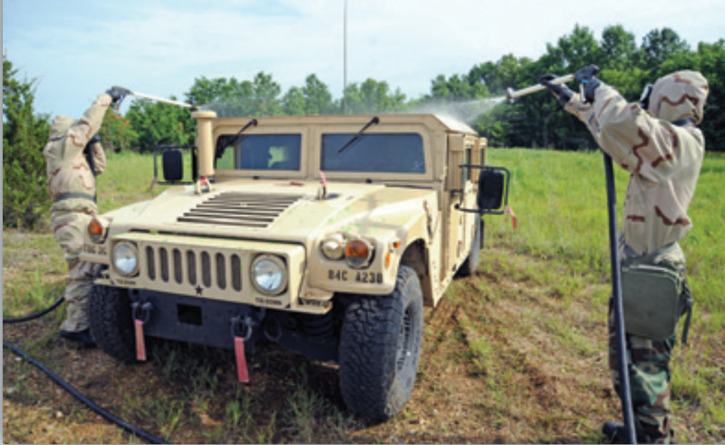
Sgt. 1st Class Antonio Diaz (left) and Pfc. Lloyd Gray of the 61st Chemical Company, 23rd Chemical Battalion at Joint Base Lewis-McChord, Wash., use an M17 lightweight decontamination system to decontaminate a humvee during day four of the competition. The pair later had to perform unmasking procedures using the M256 chemical agent detector kit, all while in mission-oriented protective posture
