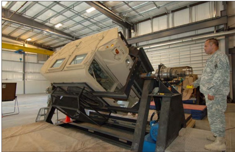
Fort Riley is only one of a handful of Army posts that have the Humvee Egress Assistance Trainers, which are helpful in training soldiers on proper techniques to use when involved in a rollover and the importance of properly securing equipment inside the humvee.
