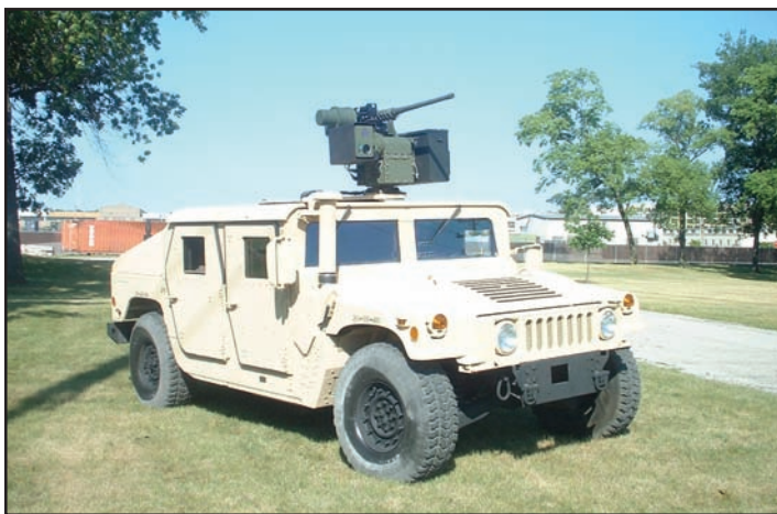
The Common Remotely Operated Weapon Station (CROWS) is a big hit with Soldiers fighting the Global War on Terrorism. The system gives Soldiers a safer way of engaging the enemy with a high first-round hit probability.
