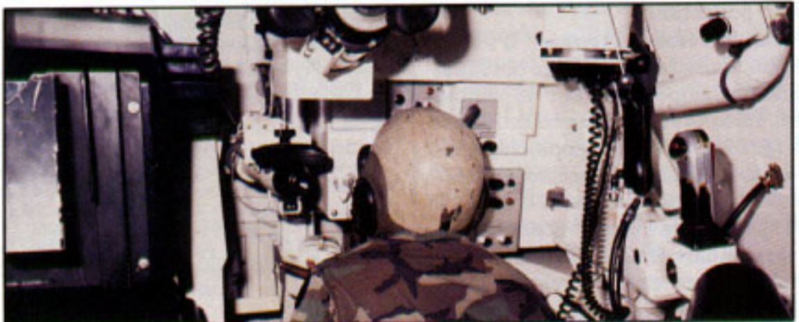
The UCFT system helps gunners acquire and identify (friend or foe) targets prior to firing.
