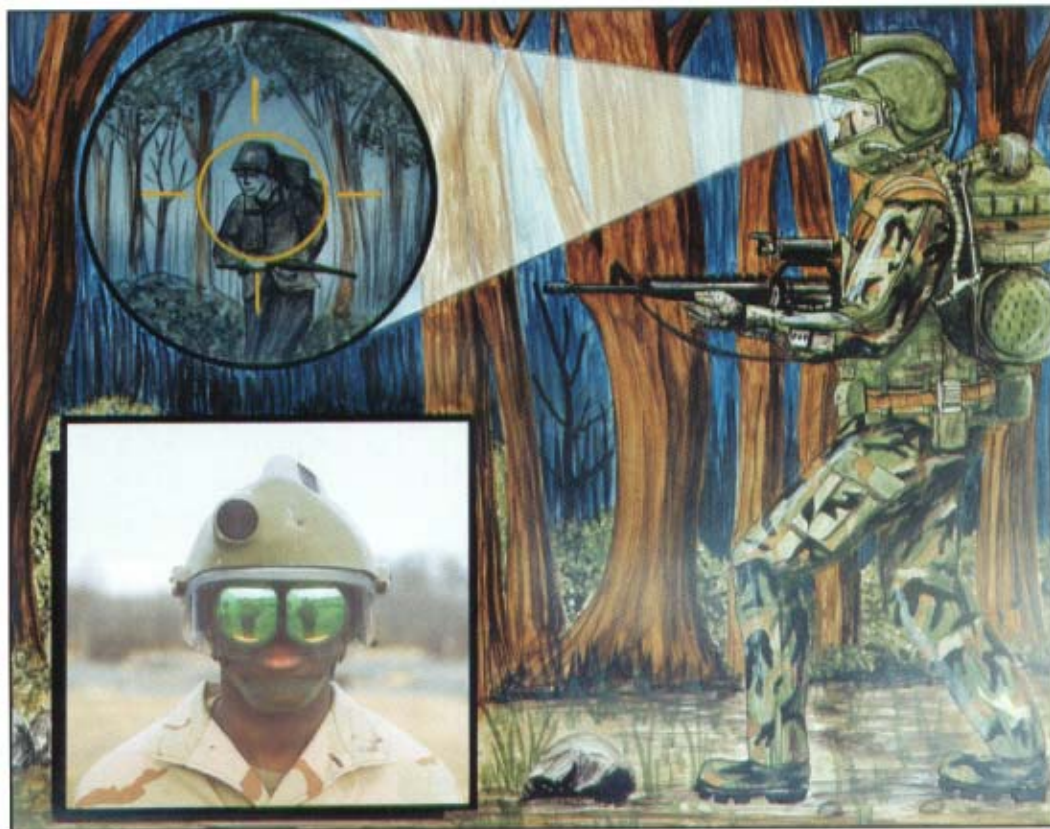
SIPE body armor and load bearing components are shown on soldier above. The SIPE weapons interface linking the weapon-mounted thermal sight to the IHS display optics for indirect viewing/firing is illustrated at right. Inset shows integrated headgear.
